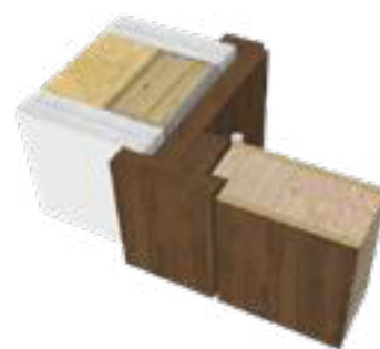
Drywall outside flush jamb with in-swing door
