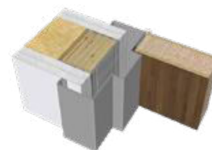
Drywall Hollow metal frame KD or welded
